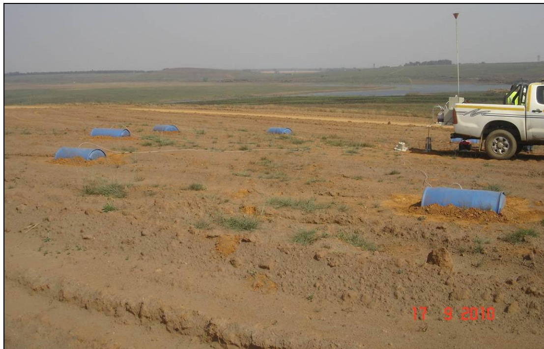
Figure 1 Typical sampling arrangement, showing half barrels and central manifold (topsoiled rehab site)
